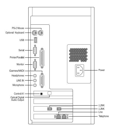
For your convenience, your computer includes USB and i.LINK connectors on both the front and back panels, allowing you to connect to either set of connectors. i.LINK connectors on the back of your system are 6-pin connectors.
